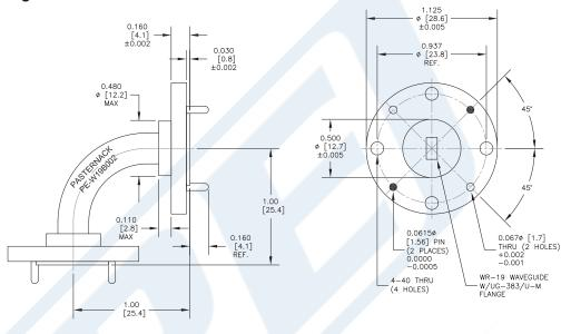
WR-19 Instrumentation Grade Waveguide H-Bend with UG383/U-Mod Flange Operating from 40 GHz to 60 GHz from Pasternack Enterprises has same day shipment for domestic and International orders. Our RF, microwave and millimeter wave products maintain a 99% availability and are part of the broadest selection in the industry.
